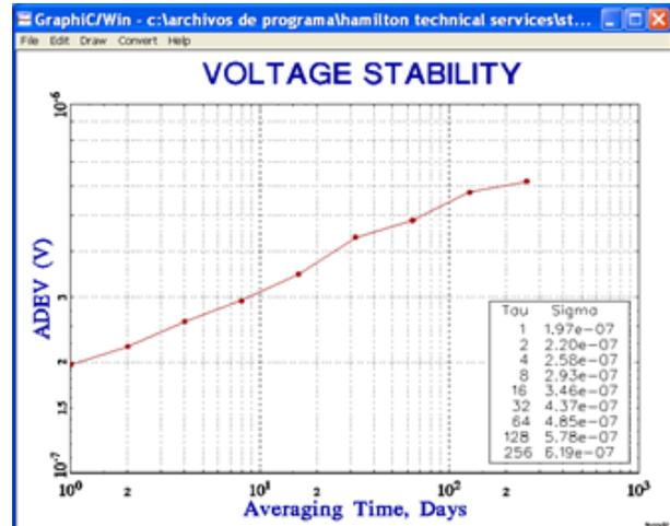
Fig. 6. Allan deviation of the voltage difference between both halves of the source, observed during six years.
