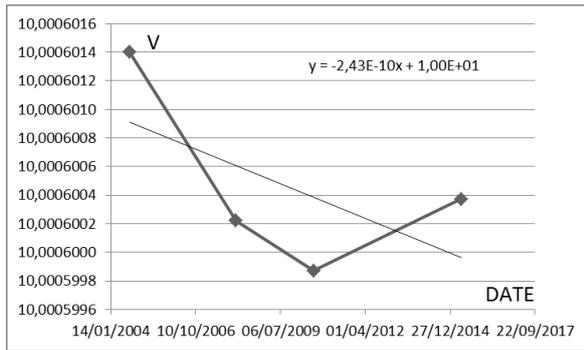
Fig. 5. Corrected voltages, subtracting the variation of the source due to repairs.
