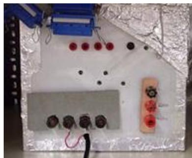
Fig. 2. First prototype of the voltage standard source.
