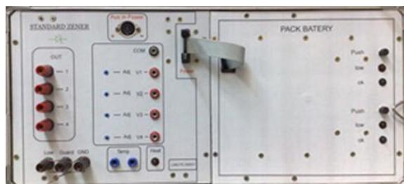
Fig. 3. Second prototype of the voltage standard.
