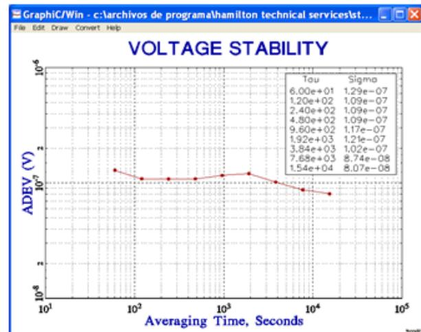
Fig. 7. Allan deviation of the voltage difference between both halves of the source, observed during one day.
