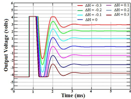
**Figure 3.** Output voltage of the GMI gradiometer obtained by computational simulations, for different magnetic field gradients  $\Delta H$ .
