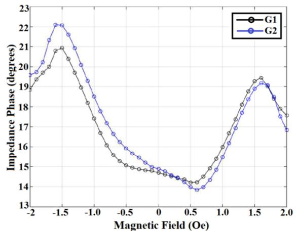
**Figure 2.** Impedance phase of both GMI samples,  $G_1$  and  $G_2$ , as a function of the magnetic field.
