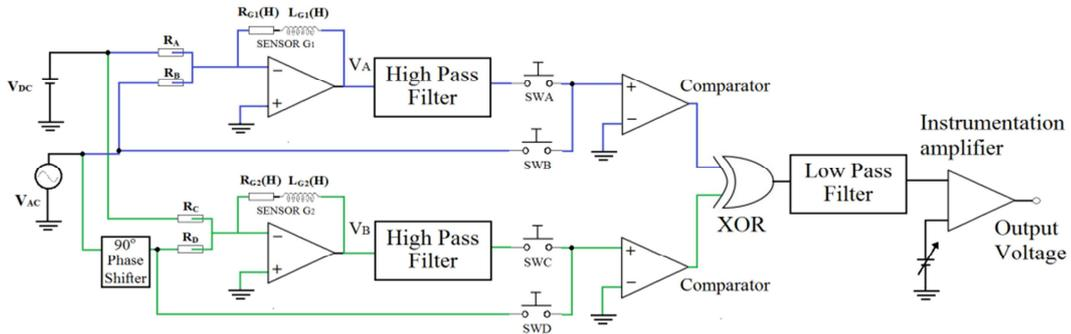
**Figure 3.** Electronic circuit of the GMI gradiometer. When SWA and SWC are closed the circuit operates as a gradiometer, when SWA and SWD are closed the circuit operates as a magnetometer using sensor  $G_1$ , and when SWB and SWC are closed it operates as a magnetometer using sensor  $G_2$ .
