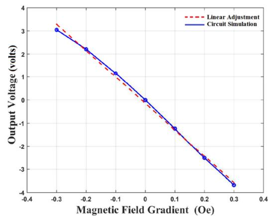
**Figure 4.** Output voltage of the GMI gradiometer as a function of magnetic field gradients  $\Delta H$ .
