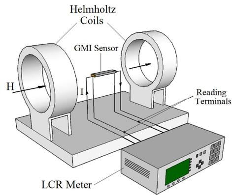
**Figure 1.** Schematic diagram of the experimental set up used to characterize the GMI samples.
