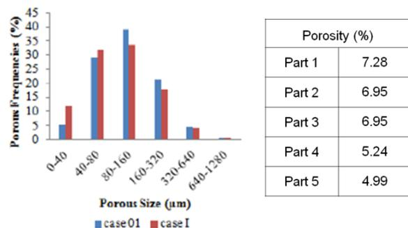
Figure 5 – Graphic of Porous frequencies VS porous size on the left and the porosity in parts during the whole sample (case I).
