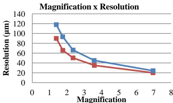
Figure 1 – Graphic of Resolution vs Magnification for detector 1120<sup>2</sup> pixel in blue and 2240<sup>2</sup> pixel in red.
