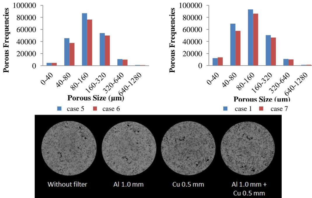
Figure 6 – Graphics comparatives of Porous frequencies VS porous size of cases 6 and 7 on the left, and cases 1 and 9 on the right. The figure below represent the same slice in different situations changing the additional filter.
