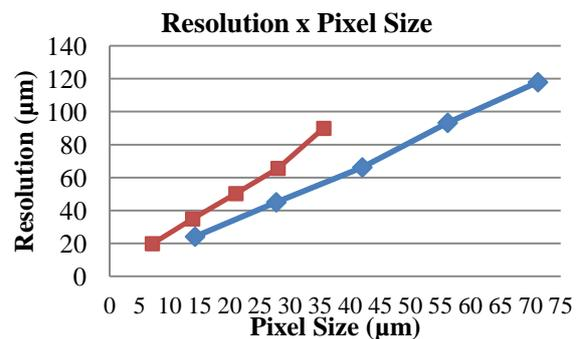
Figure 2 –Graphic of Resolution vs pixel size for detector matrix 1120<sup>2</sup> pixel in blue and 2240<sup>2</sup> pixel in red.
