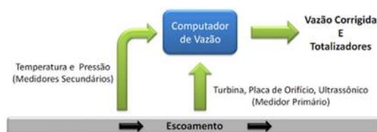
Figura 1: Typical flow computer connexion to a pipeline and a flow measurement system.
