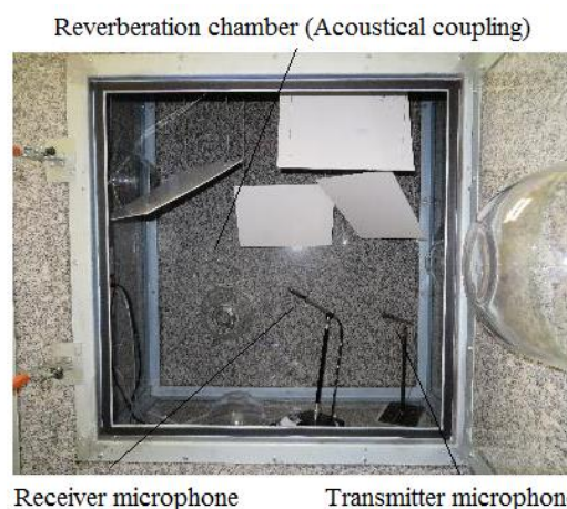
Figure 4. Experimental arrangement for diffuse-field reciprocity calibration in Inmetro.
