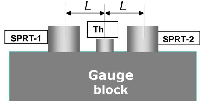
Fig.7. Thermometers configuration for precise calibration, and precise temperature measurement of a particular point on the GB surface.
