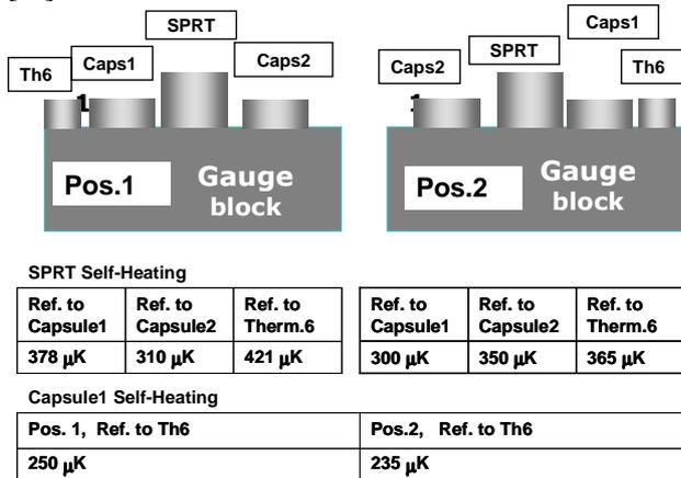
Fig.4. Results of the first experiment on the SH measurements on the gauge block surface.
