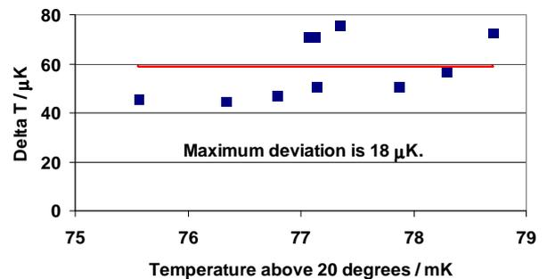
Fig.8. Measurements of an axial temperature variation on the GB surface inside interferometer.
