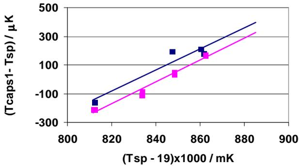
Fig.5. Demonstration of the variation in the GB temperature distribution, caused by measurement current in capsule PRT.
