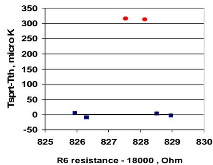
Fig.3. Self-heating measurement in DDS, using double-channel technique.
