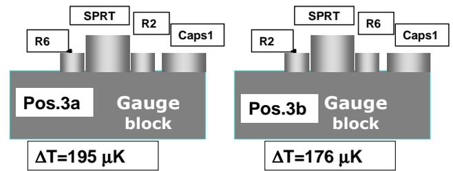
Fig.6. Results of the last experiment on the SH measurements on the gauge block surface.
