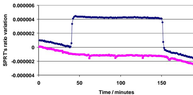
Fig.1. Variation of the temperature regime of the equalizing block in DDS with the increase of the measurement current in the SPRT.
