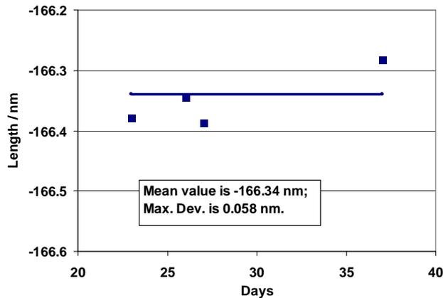
**Fig.9. Demonstration of the time stability in length measurements of a 100 mm steel GB at the level of 0.058 nm.**
