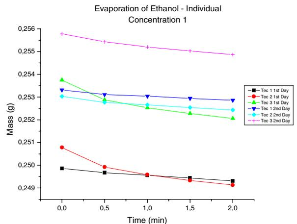
Figure 1: Evaporation experiment for concentration 1 by the individual methodology.
