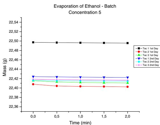
Figure 10: Evaporation experiment for concentration 5 by the batch methodology.
