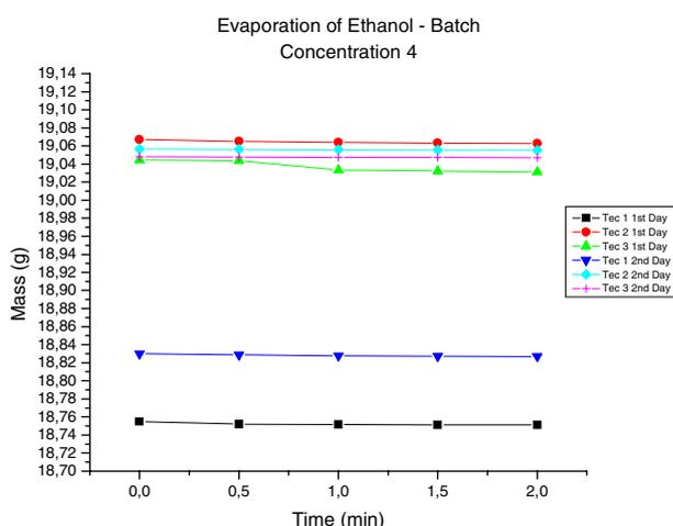
Figure 9: Evaporation experiment for concentration 4 by the batch methodology.
