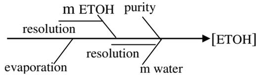
Scheme 1: Cause and effect diagram for the determination of the measurement uncertainty inherent to the characterization of the concentration of ethanol in water.
