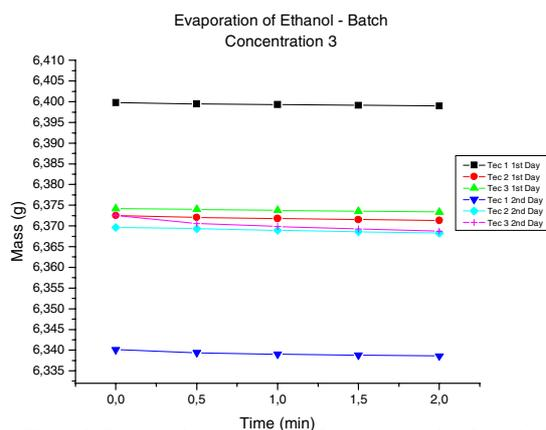
Figure 8: Evaporation experiment for concentration 3 by the batch methodology.
