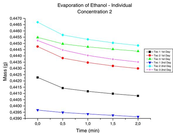
Figure 2: Evaporation experiment for concentration 2 by the individual methodology.
