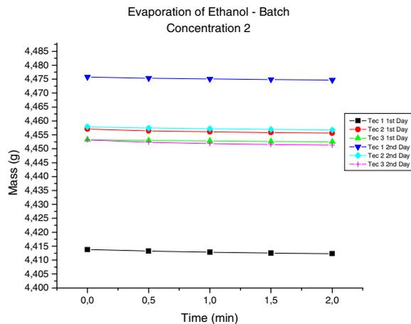
Figure 7: Evaporation experiment for concentration 2 by the batch methodology.
