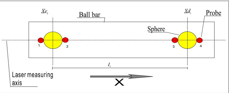
Figure 3 - Probe positioning, relative to spheres.
