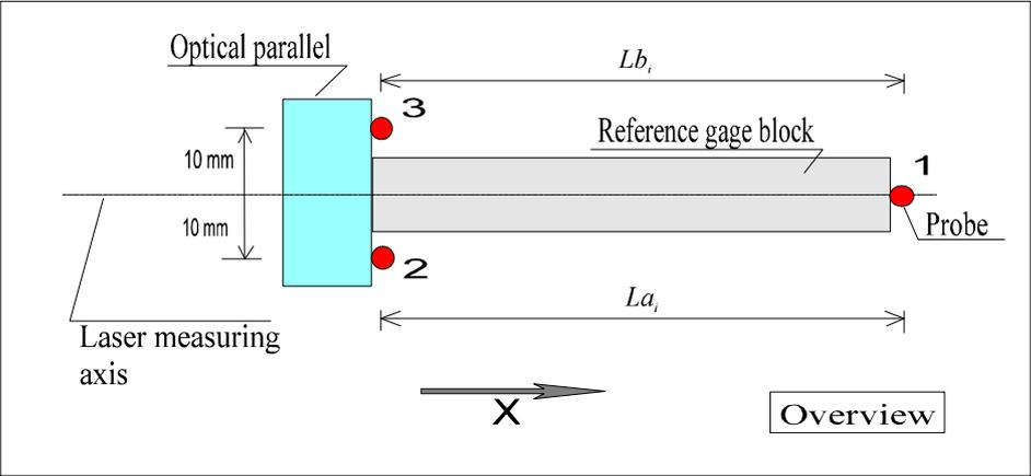
Figure 2 - Probe positioning in the gage block measurement.
